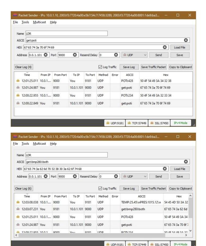
Now simply enter the requests that the ESP32 would otherwise send by hand in ASCII. Send sends the data to the ESP8266. If you get the right answers, then this part of the project will also work. Otherwise you still have the emergency brake to touch up the program.
