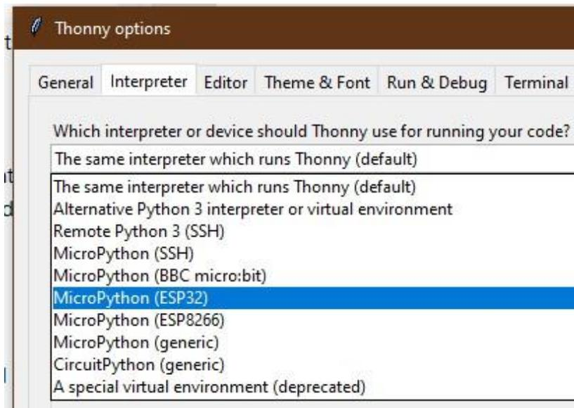
Now download the Micropython firmware for the ESP32 and save this file in a directory of your choice. The bin file must first be transferred to the ESP32. This also happens to Thonny. Call up Thonny Options again with Run - Select Interpreter.... At the bottom right click on Install or update Firmware.
