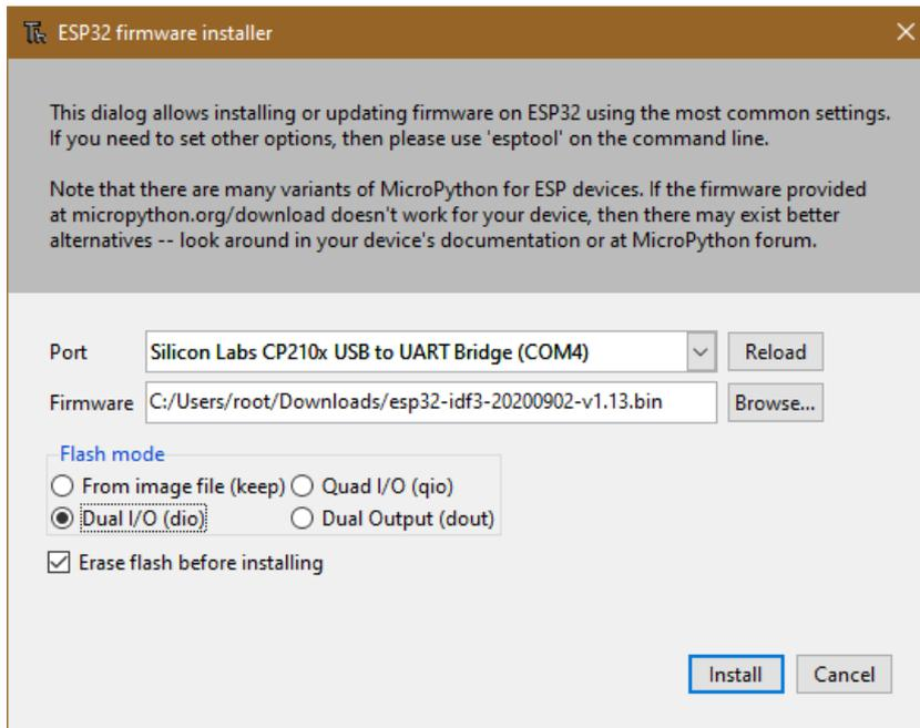
Select the serial port to the ESP32 and the downloaded firmware file. Start the process with Install. After a short time, the MicroPython firmware is on the controller and you can send the first commands to the controller via REPL, the MicroPython command line. For example, enter the following command in the Terminal window.
