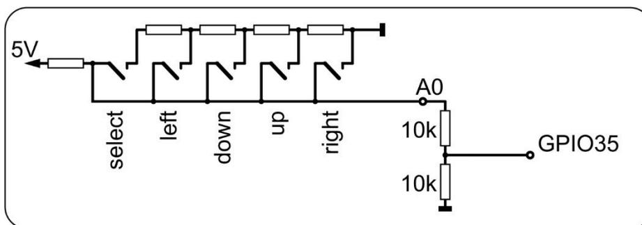
The buttons SELECT, LEFT, UP, DOWN and RIGHT are connected to a resistor cascade, which in turn is connected to 5V at the hot end. The buttons apply the respective level to connection A0 of the keypad, which therefore carries 5V when idle. We halve the voltage applied here using a voltage divider made up of two 10kΩ resistors to a tolerable 2.5V. We connect the center tap to the analog input GPIO35 of the ESP32. We are making further adjustments in the KEYPAD class.
