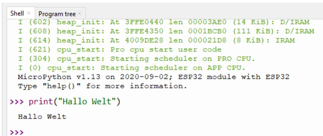
In contrast to the Arduino IDE, you can send individual commands to the ESP32 and, if it is MicroPython instructions, it will respond well. On the other hand, if you send a text that the MicroPython interpreter cannot understand, it will alert you to this with an error message.
