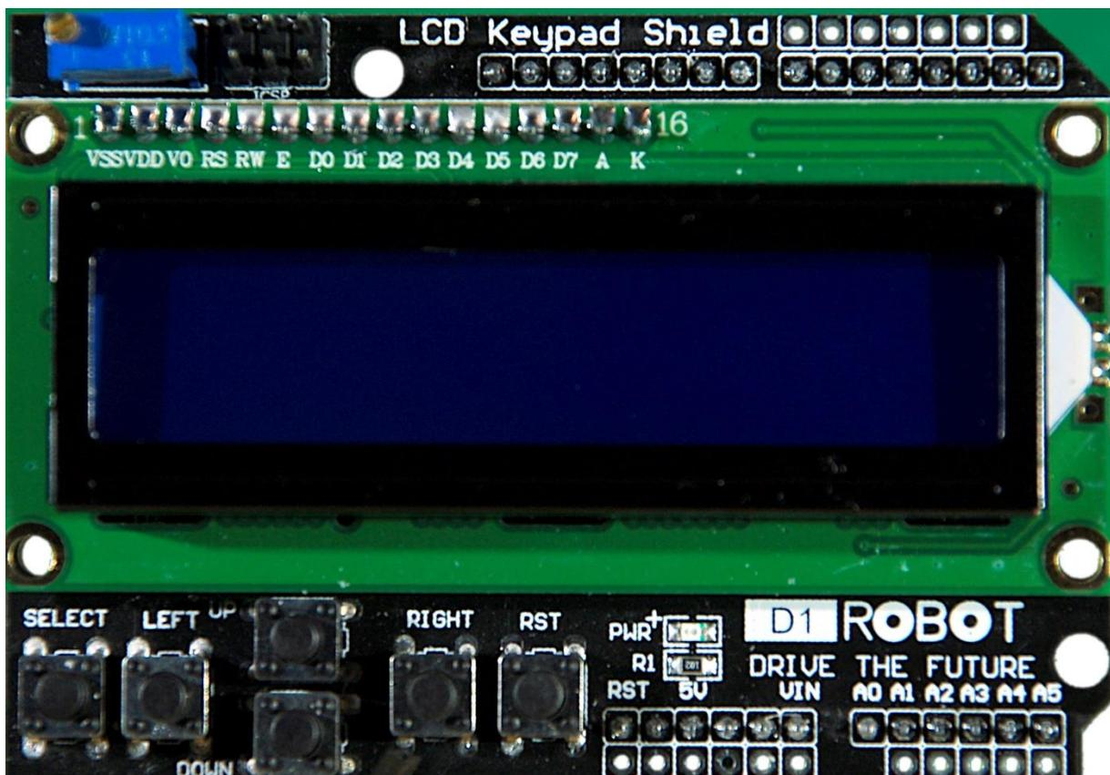
In addition to the 16x2 representation, the display with keypad offers a total of 6 keys, five of which have a control function in the current project. These buttons supply the voltage from the nodes of a resistor cascade to an ADC input (GPIO35). The levels are decoded by the ESP32 and assigned to various actions. You will learn more about this later.
