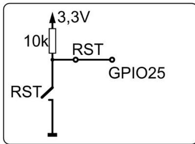
If you solder a wire to the hot connection of the start button on the underside of the SIM808 board as in the following figure, you can switch on the module from the ESP32 with a pulse of one second duration. This can be done while booting, as I did in my program. In the idle state, the line is at 3.3V, so the pulse must be against GND. The module is switched off again with a pulse of more than 3 seconds.
