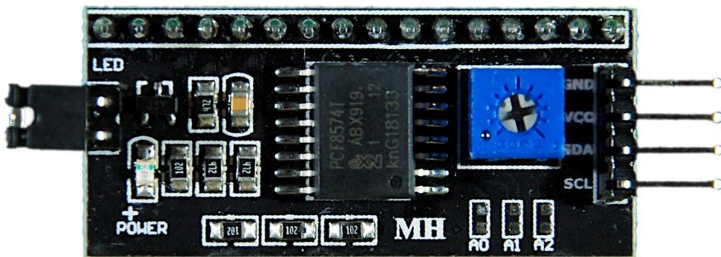
Its inputs are 3.3V-compatible and the outputs can handle the 5V from the display. To connect to the ESP32, only 2 lines, SCL (21) and SDA (22) are now required instead of the 6 direct connections. The I2C bus is also available to other sensors, such as a BMP / BME280, which is intended as an extension of the circuit.
