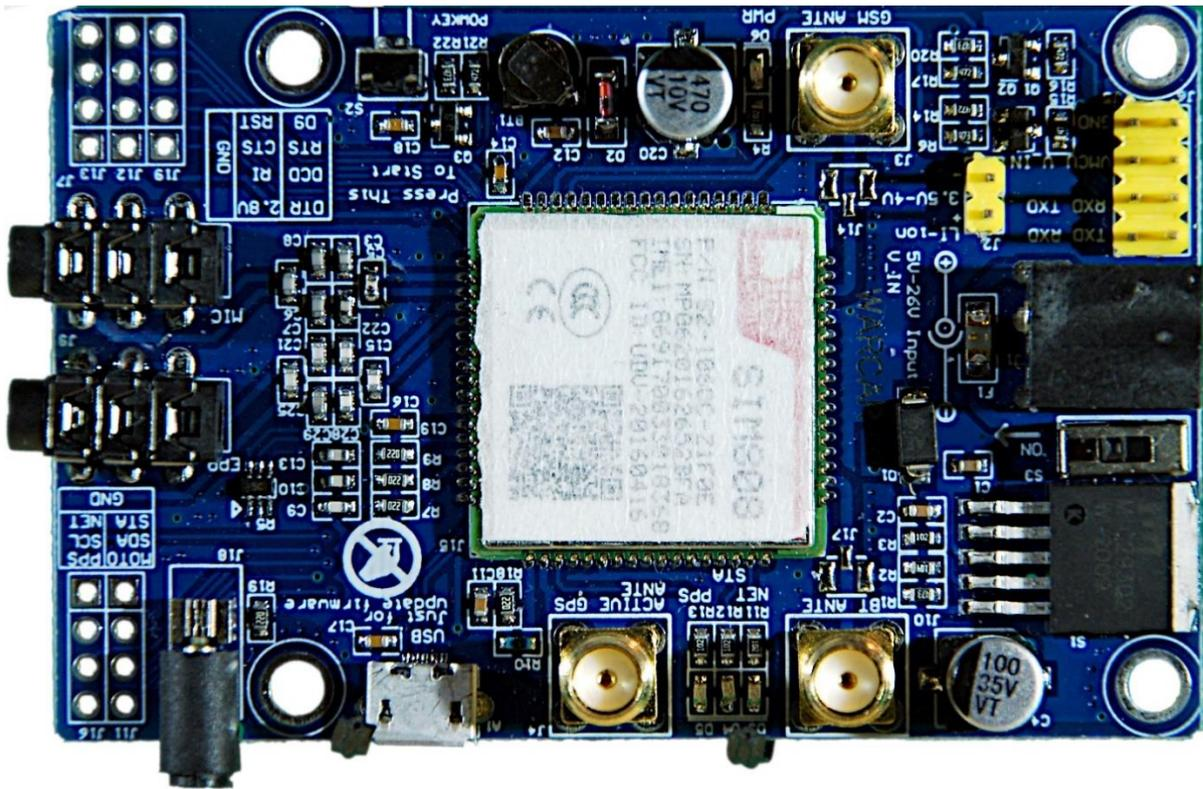
There remains the SIM808. It is normally supplied with voltages of 5..12V via the pipe socket (2.1x5.5), but it also offers a connection for 3.5 to 4.2V for a lithium cell. A connection next to one of the GND pins is available on the yellow pin header for external 5V. On the larger yellow pin base on the top left is GND and exactly below + 5V Vin.
