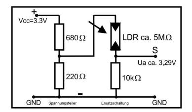
The calculation of the voltage between the resistors of  $680\Omega$  and  $220\Omega$  gives a value of 1.07V.
