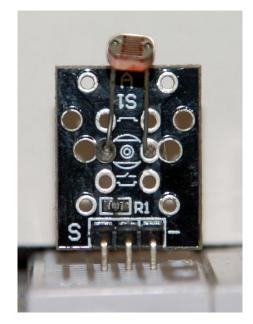
If you stick to the labeling on the circuit board, the positive connection is in the middle and the GND connection is on the right-hand pin labeled "-". This corresponds to the circuit diagram above.
