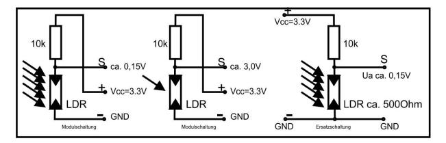
Pay close attention to the voltages and polarities indicated in the sketches. The number of arrows shows the intensity of the incident light. In addition to the LDR, the board contains a fixed resistor R1 of 10kOhm, which is connected in series with the LDR. This circuit is also known as a voltage divider circuit because the voltage that can be measured between the two resistors is always lower than that which is applied to the ends of the circuit. There are two connection options for the PCB.
