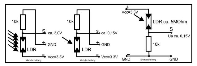
To explain the behavior of this circuit, I'll take a quick look at physics and math. According to what is commonly referred to as Ohm's law, the voltage U applied to a conductor and the strength I of the current flowing through it are directly proportional to one another. The quotient U / I is therefore a constant (which one likes to define as electrical resistance). This helps us to roughly calculate what to expect. The resistor R1 on the board has a fixed value of 10kOhm = 10000Ohm.
